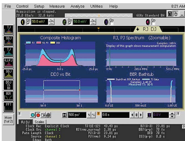
Figure 12. Low frequency jitter measurement using EZJIT Plus
